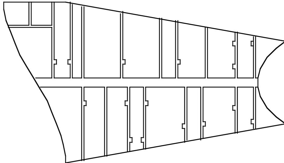
Plating detail along the main cockpit tube. This represents only the upper surface plating up to the tube bend. Detail along the spine is omitted.
